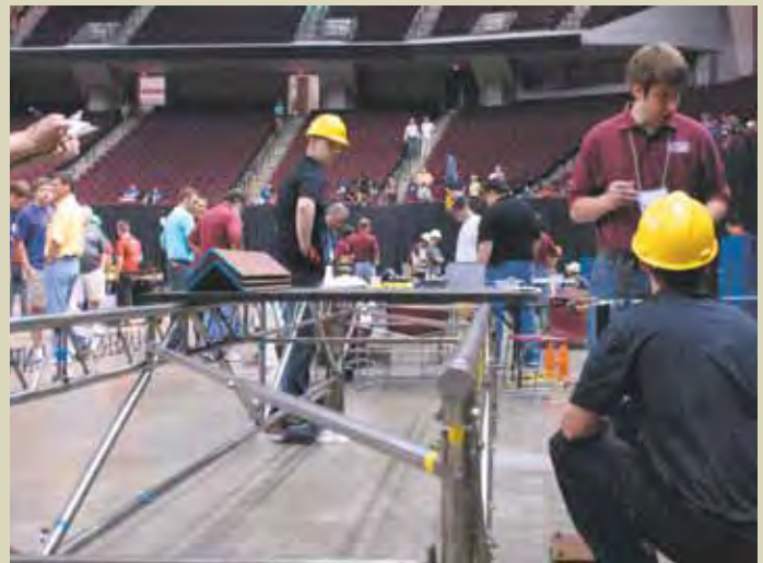
Measuring the Lakehead University bridge's horizontal deflection
