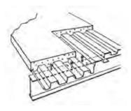
Figure 2 Deck perpendicular to beam
