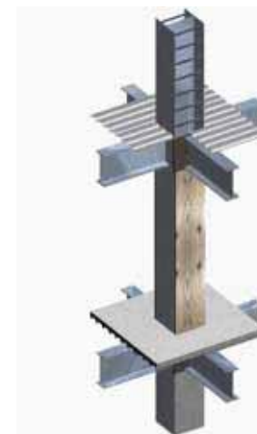
Composite action / columns: The partially encased thin-walled built-up section is the newest addition available to designers (see CSA S16-01 Clause 18.3). This variation is particularly attractive for multi-storey buildings and has been the subject of substantial research in Canada at École Polytechnique and the University of Alberta. The end result is a composite column that is very efficient, with steel and concrete acting compositely and sharing the load about equally.
